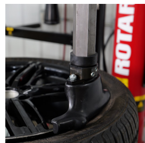
SHOWN: Helper arm demounting lower bead
