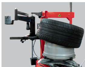
SHOWN: Helper arm demounting lower bead
